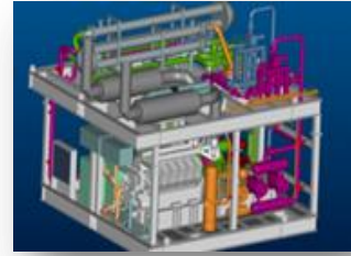
Figure 3 example of compact piping layout on an FPSO
