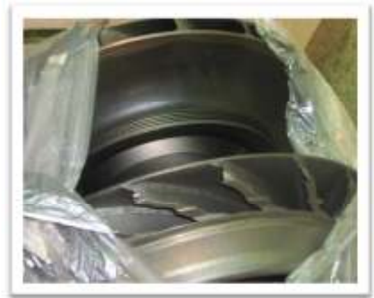
Figure 1: Centrifugal Compressor Damaged During Surge Event
